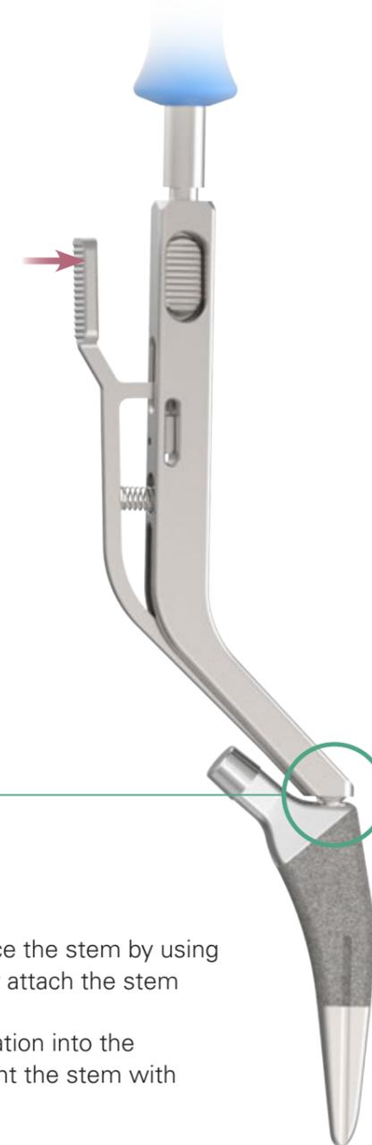
After trial reduction, remove the broach and introduce the stem by using the **Quick Connect Holder**. Use the holder to firmly attach the stem via the insertion hole on the stem shoulder. Gently tap the holder to achieve initial stem implantation into the medullary canal. Proper care should be taken to orient the stem with proper alignment and version.
